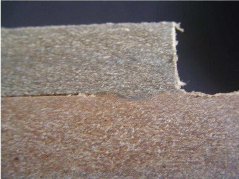
Figure 8. Magnified view of energy director area of bonded material
