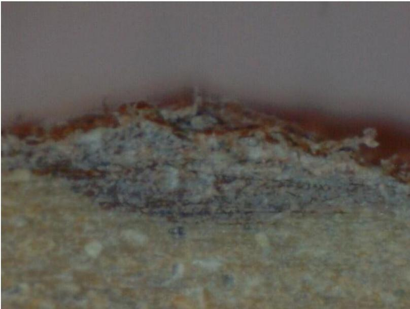
Figure 10. Magnified view of pull separation of welded material.
