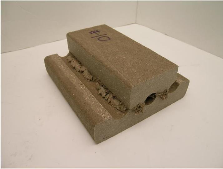
Figure 1. Weyerhaeuser Chiocedek Premium deck boards manufactured by Advanced Environmental Recycling Technologies (A.E.R.T.) Vibration welded Shows example of flash when weld is close to the edge.
