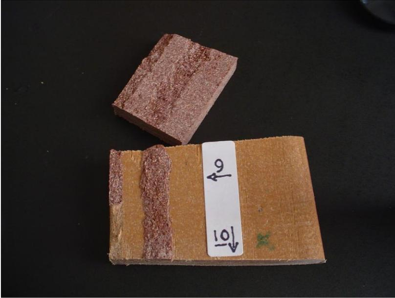
Figure 7. Show material bond at weld line after pull separation
