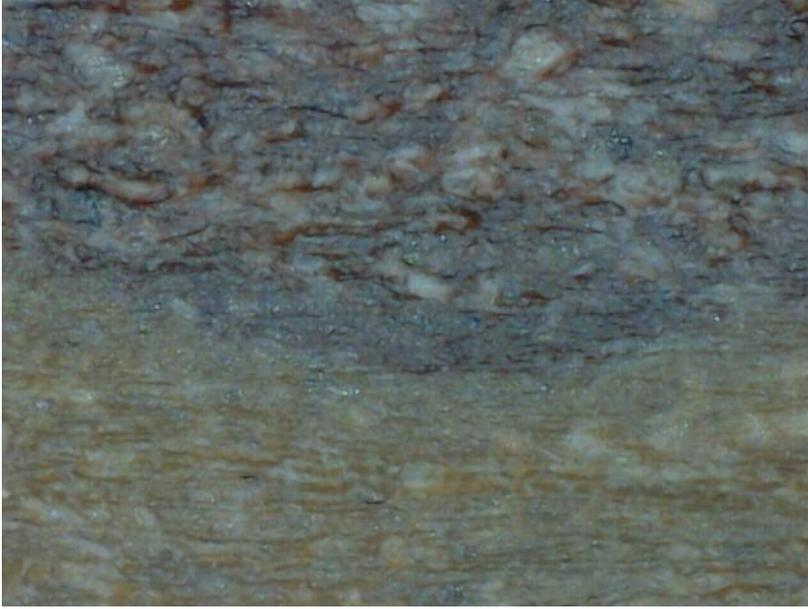
Figure 9. Magnified view of welded Wood Composite material. Shows molecular intertwine of polymer at energy director area.
