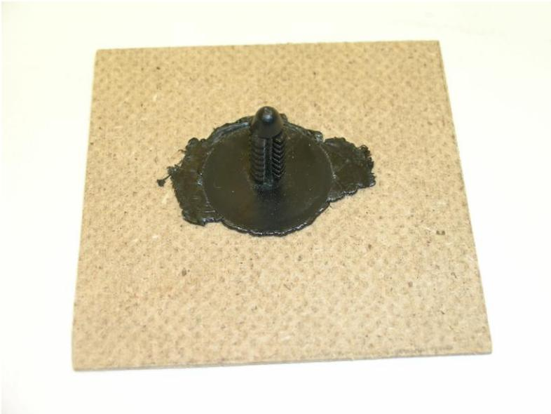
Figure3. Polypropylene injection molded fastener attached to off the shelf chipboard samples Injection molded
