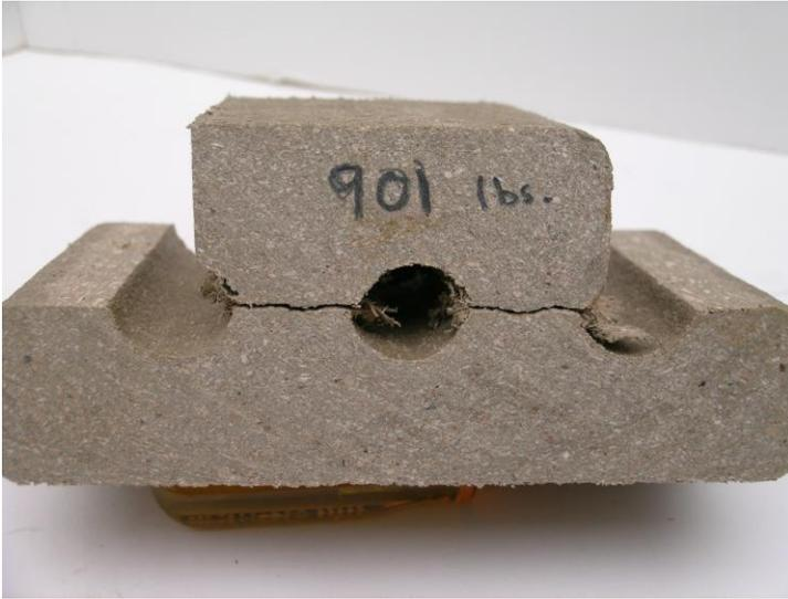
Figure 11. Shows fracture area of sample pulled material
