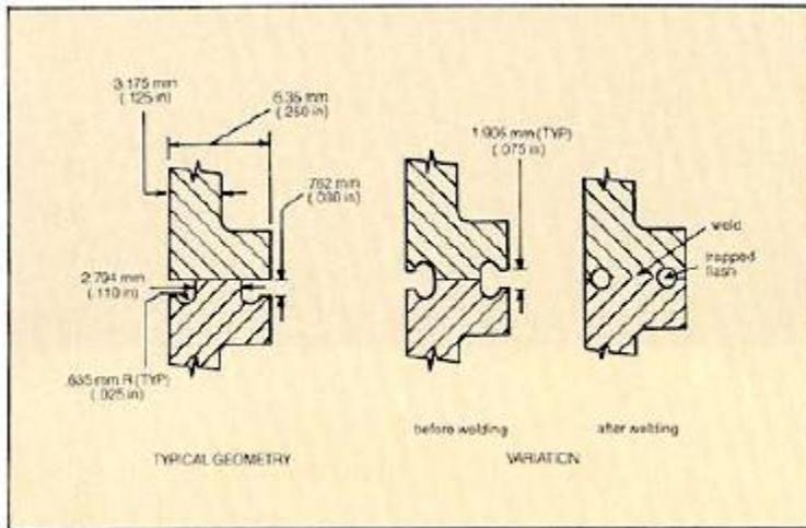
Figure 5. Typical vibration weld energy director design (Dupont)
