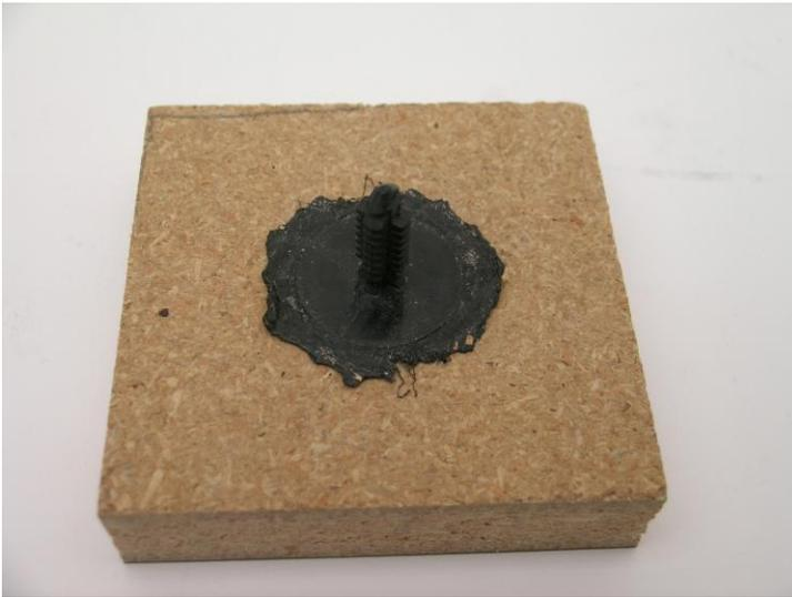
Figure2. Polypropylene injection molded fastener attached to off the shelf chipboard samples Injection molded
