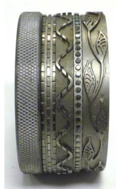
Figure 5: Patterns used to weld film or fabric
