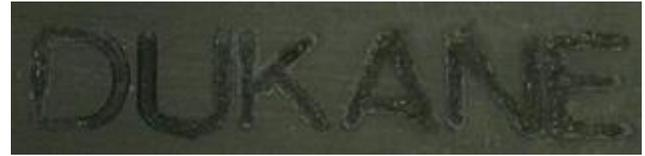
Figure 14: Laser over-welding causes burns at the joint
