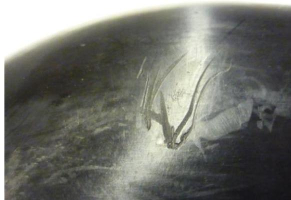
Figure 9: Spin welding tooling marks
