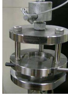
Figure 5. Custom pull test fixture.
