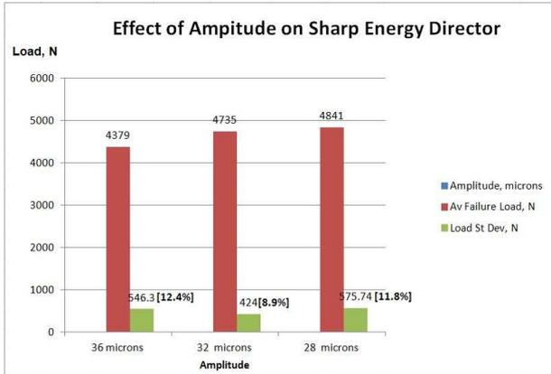
Figure 11. Sharp ED. Average Failure Load and Standard Deviation as a Function of Amplitude. Standard Deviation percentages in bold.
