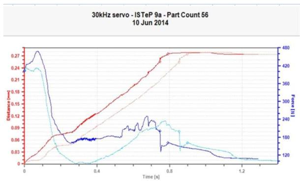
Figure 19. Force Distance Diagram for No Melt Detect Setting (darker red and blue lines) compared to Melt-Detect™ at 2% (lighter red and blue). Velocity Profile of 0.25 to 0.40 mm/sec.
