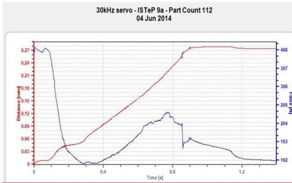
Figure 14. Typical Force Distance Diagram for Welds Produced with Weld Velocity Profile 0.25 to 0.40 mm/sec.
