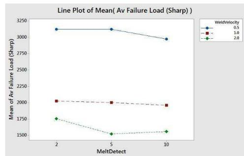
Figure 8A. Sharp ED: Melt-Detect™ vs. Ave. Failure Load.
