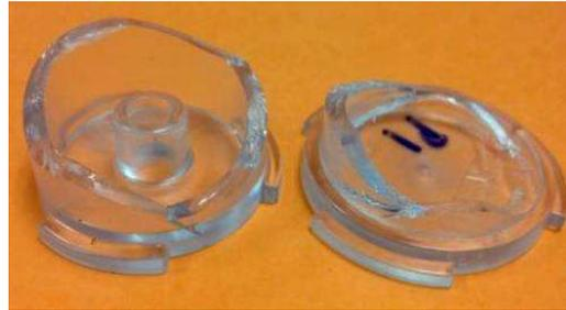
Figure 16. Welded sample broken through parent material.
