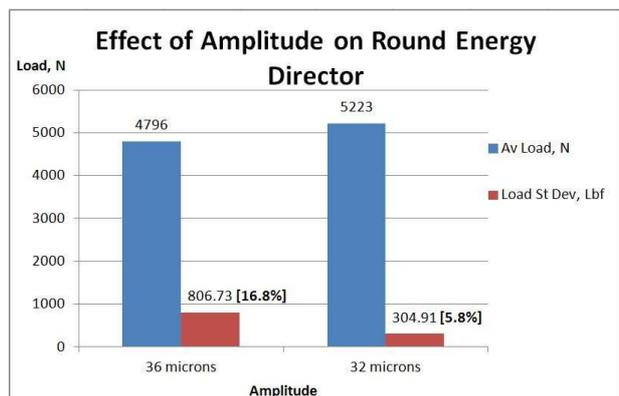
Figure 10. Round ED: Average Failure Load and Standard Deviation as a Function of Amplitude after Weld Velocity was Optimized. Standard Deviation percentages in bold.
