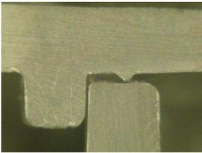
Figure 3. A cross-section of a 90° ED on an ISTE P part prior to welding.
