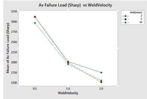
Figure 7A. Sharp ED: Weld Velocity vs. Ave. Failure Load.
