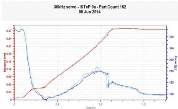
Figure 18. Force Distance Diagram for Melt-Detect™ at 10% Compared to Reference 2%, Velocity Profile 0.25 to 0.40 mm/sec,
