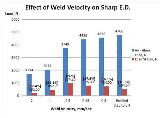
Figure 12. Sharp ED Ave. Failure Load as a Function of Weld Velocity. Standard Deviation percentages in bold.
