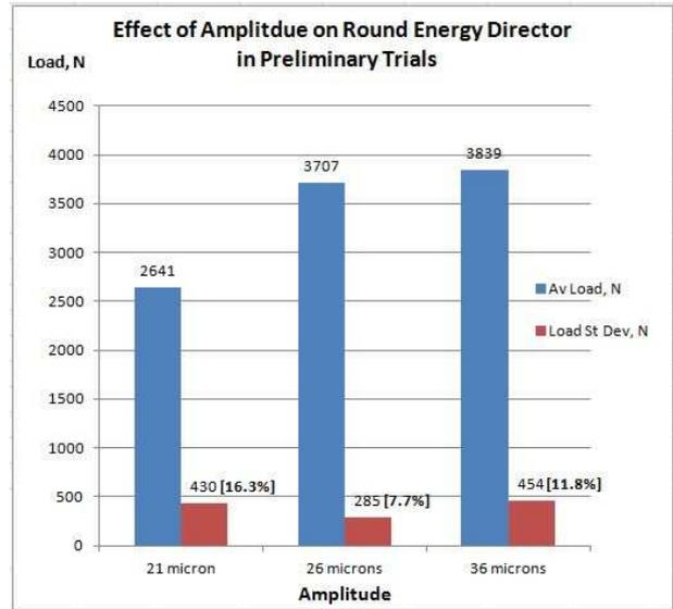
Figure 9. Average Failure Load and Standard Deviation as a Function of Amplitude in Preliminary Trials. Standard Deviation percentages in bold.
