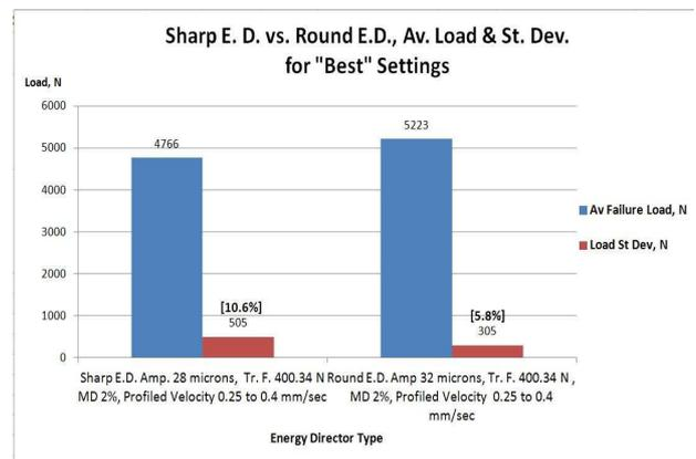
Figure 20. Best Average Failure Load and Standard Deviation results generated for sharp and round EDs. Standard Deviation percentages in bold.
