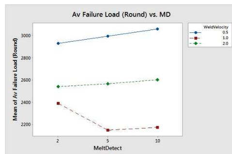
Figure 8B. Round ED: Melt-Detect™ vs. Ave. Failure Load.
