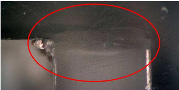
Figure 15. Melt layer image for weld velocity profile 0.25 to 0.4 mm/sec. Note the large homogenous area encircled.
