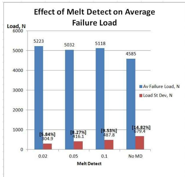
Figure 17. Av Failure Load as a Function of Melt-Detect™ Setting. Velocity Profile 0.25 to 0.4 mm/sec. Standard Deviation percentages in bold.
