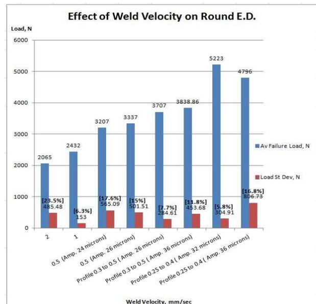
Figure 13. Round E-D. Average Failure Load as a Function of Weld Velocity. Standard Deviation percentages in bold.
