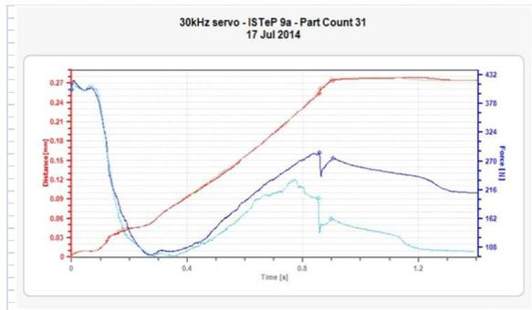
Figure 21. Comparison of Force Distance Diagram for sharp (dark blue) and round (light blue) EDs Welded Using Weld Velocity Profile 0.25 to 0.40 mm/sec
