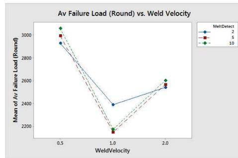
Figure 7B. Round ED: Weld Velocity vs. Ave. Failure Load.
