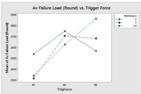
Figure 6B. Round ED: Trig. Force vs. Ave. Failure Load.
