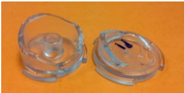
Figure 7. Typical tensile failure through parent material.
