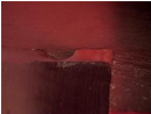
Figure 3. A cross-section of a round ED on an ISTeP part prior to welding.
