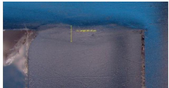
Figure 8. Constant weld velocity of 1.0mm/s. Melt penetration 361 microns. Average Failure Load 2432 N.
