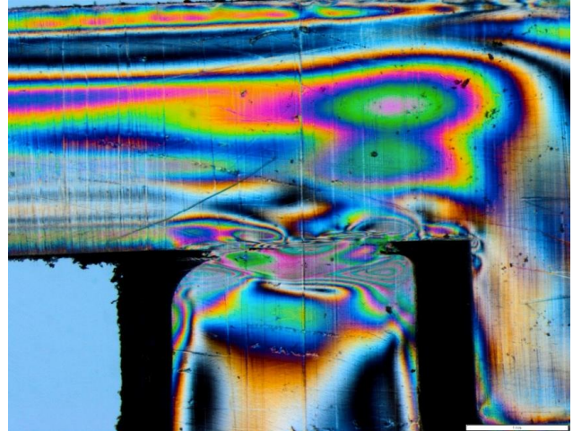
Figure 11. Melt Zone Image for Sample Welded with Weld Velocity 1.0 mm/sec photographed in polarized light.
