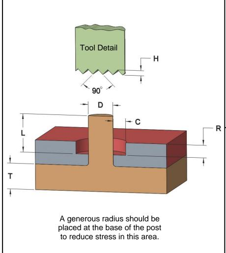
The knurl staking configuration is generally used on parts that have an unusual post shape or when alignment will be difficult.
