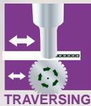
**Ultrasonic Slitting:** When a thermoplastic material is slit ultrasonically, its edges are also sealed, preventing the fibers/yarns from unravelling. The smooth, beveled edges also prevent the buildup of roll material.
