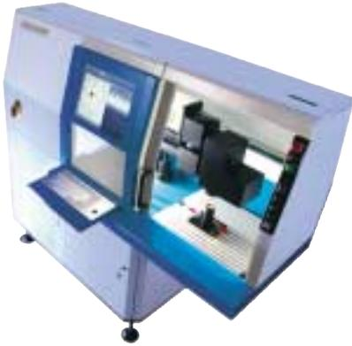
Laser welding requires the absorption of laser light. One material transmits the coherent laser light and the other material absorbs the light and converts it to heat. Parts that appear to be black to the human eye can be transparent or opaque at the wavelength of the laser light. Clear-to-clear joints and joints that are optically transparent can be readily achieved by use of special coatings.
