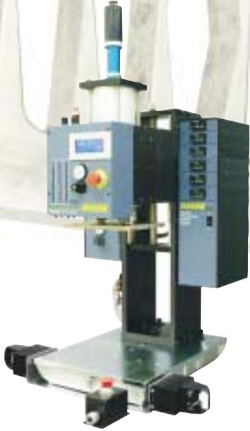
Our **Thermal Presses** can handle multiple stake posts or inserts on multiple planes simultaneously. These machines can be used for date coding, embossing or degating.
