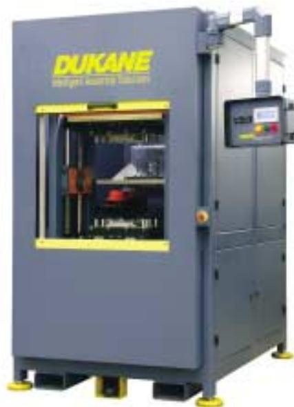
Dukane **Spin Welders** can handle almost any part you can imagine that has a circular joint. Highly reliable hermetic seals and maximum flexibility in part fixturing are just two advantages that spin welding has to offer.
