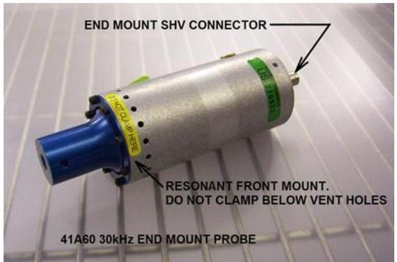
welding pressure and design of the interface. Because of these concerns, **DO NOT** clamp within 1" (25mm) of the front of the housing. This will not be a problem if you secure the probe near the back of the housing.
