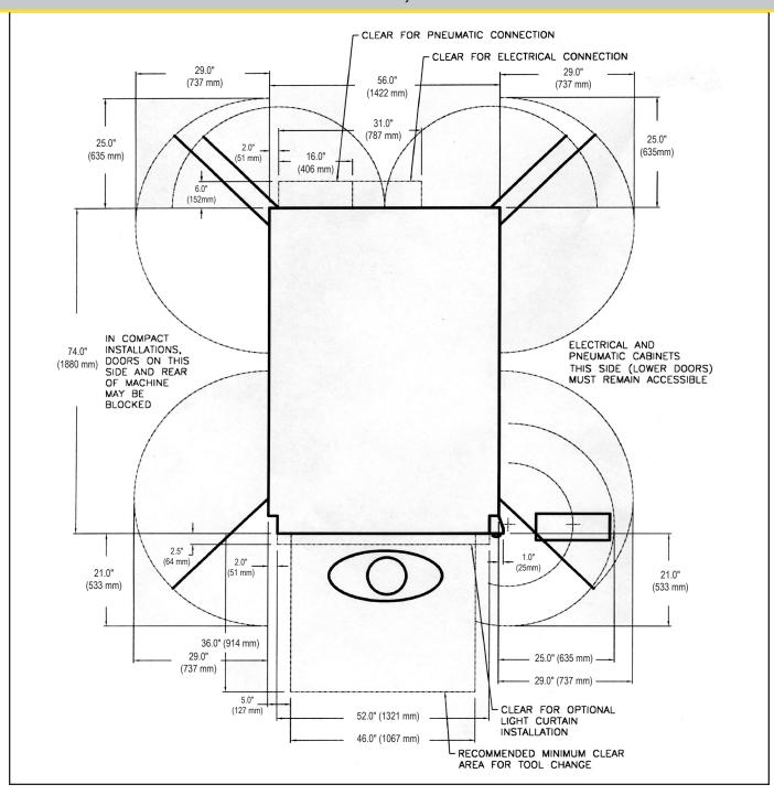
Electric Service Required: 240 V, 3 phase, 20 amps Pneumatic Service Required: 75 to 90 psi (5-6 bar)
